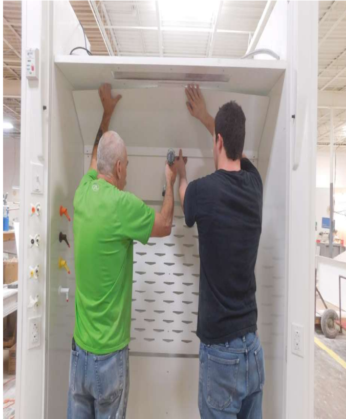
Install baffle to back wall. Secure with #10 x 3/4" sheet metal screws and PVC caps.
