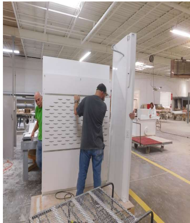
Install the Right Side Wall to the Back Wall, with provided #8 or #10 sheet metal screws.
